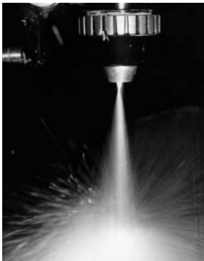
Thermal spray of protective coating onto steel substrate.
