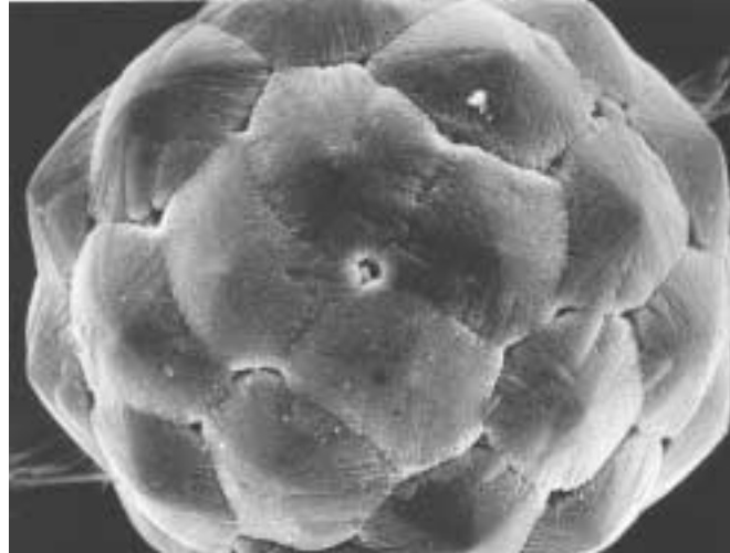
A resolidified alumina particle that demonstrates dendritic growth.
