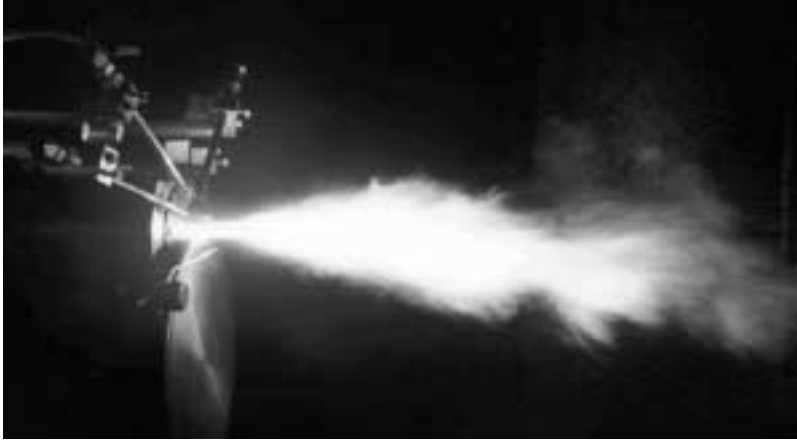
Plasma spraying of ceramic onto a material to be protected from high temperatures.
